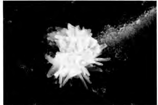
Fig. 5. A photomicrograph of alteration that occurs on the bottom surface of glass that has been in contact with the weld-affected ss. Magnification 3000X.
