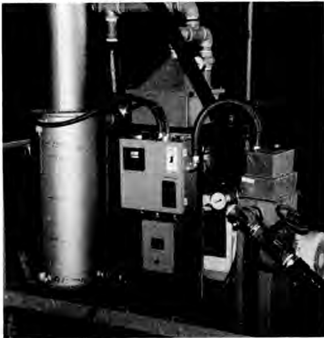
Fig. 2. The dewatering test skid.
