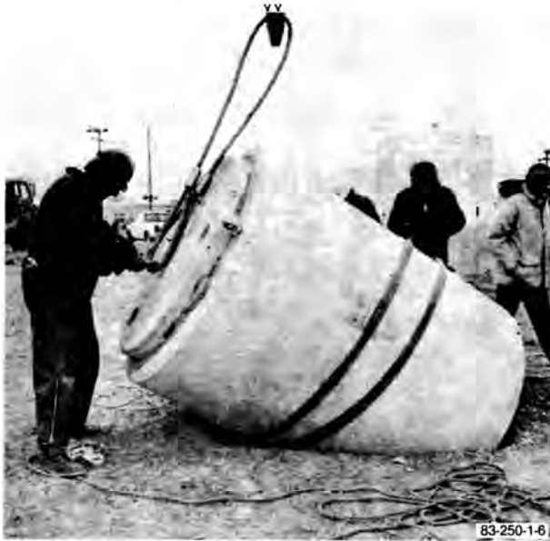
Fig. 7. The High Integrity Container after being dropped from 25 feet onto a yielding surface at INEL.
