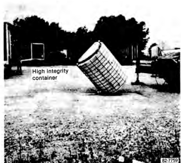
Fig. 6. Drop test of the High Integrity Container showing drop-test setup (A) and instant of impact (B).
