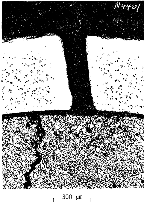
Fig. 1. Metallographic Section of a Laser-Drilled Cladding Defect After 60-Days Test Duration. No visible attack of the fuel by the leaching solution was observed. (Etched to reveal fuel microstructure.)
