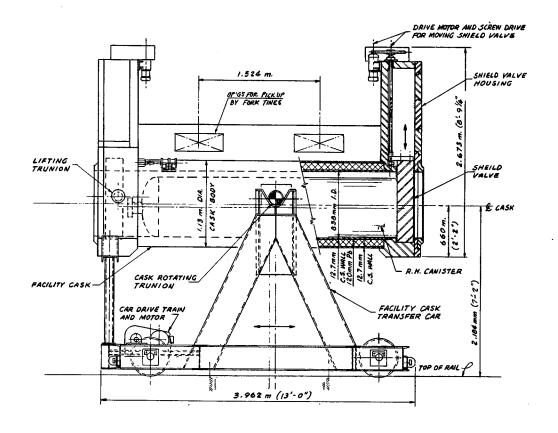
Fig 3. Facility Cask on Transfer Car.
