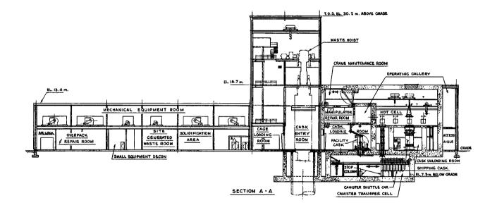
Fig 2. Waste Building Elevation.
