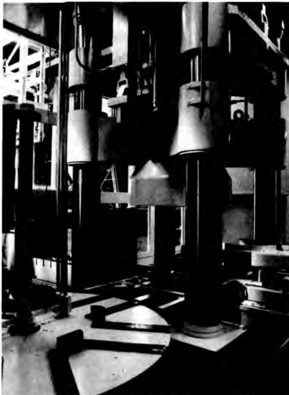
Fig. 3-Photograph of 1500 tons hydraulic press. Note entry of drum through air-lock.
