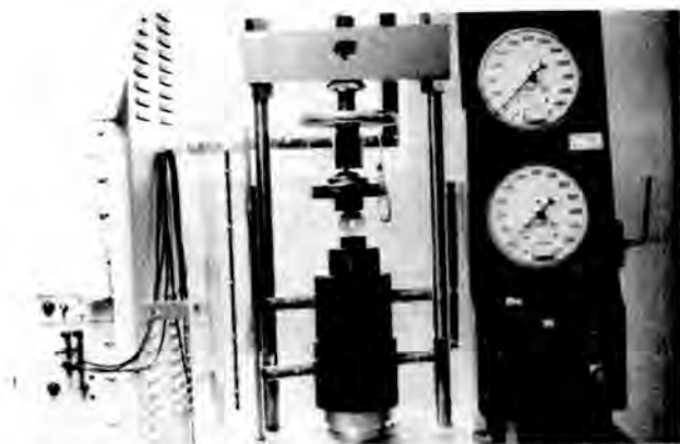
Fig. 4. Test set-up for ring tension test.
