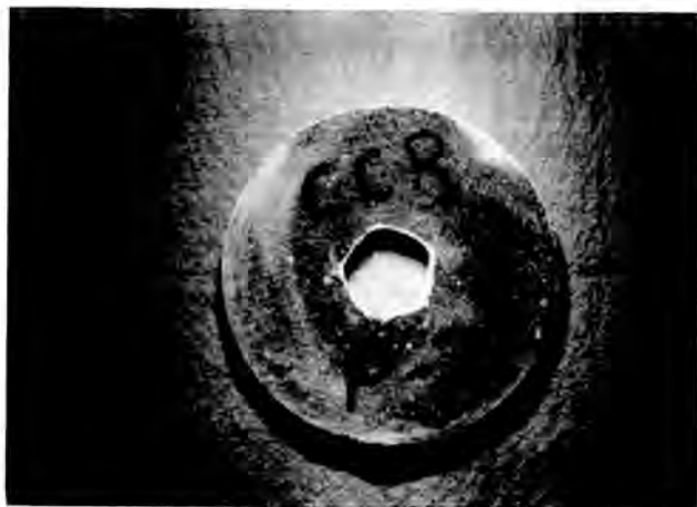
Fig. 3. Sample of fine grained Catalina Granite treated with penetrating dye. Note the damage zone, enhanced by the dye, particularly visible on the upper (in photograph) periphery of the hole. The above 6-inch diameter disk contains an overcored 1 1/2-inch percussion drilled hole, with a frequently observed pentagonal shape.
