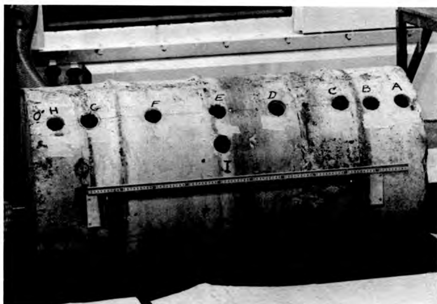
Fig. 6. Side view of the concrete waste form showing the core hole locations along the 0^{\circ} and 20^{\circ} longitudinal axis.
