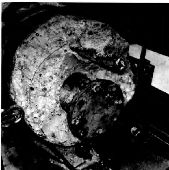
Fig. 7. View of the exposed flange end of the inner steel container.
