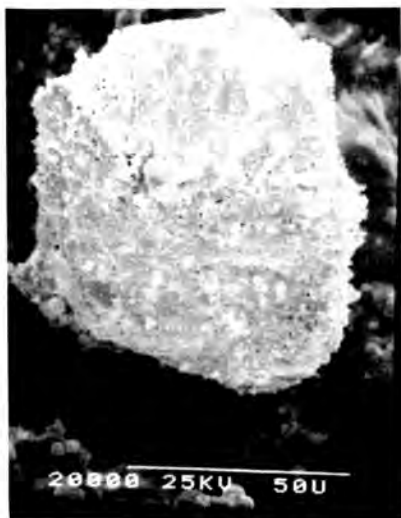
Fig. 6. A SEM photograph of a time-integrated aluminum planchet sample showing a 70 \mu\text{m} geometric diameter \text{UO}_2 particle.
